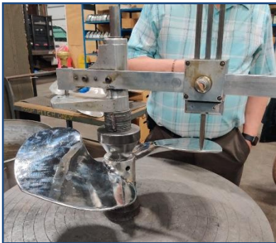
50HP Sample Prop Wet Testing and QC Inspections at AAS
