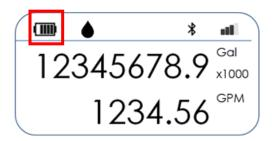
The meter continuously monitors battery life. When the battery power is low, the battery cell icon will show an empty battery. Battery replacement is required at this time.
