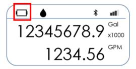
When the meter detects an empty pipe, the meter will stop measuring and display an empty droplet symbol.
