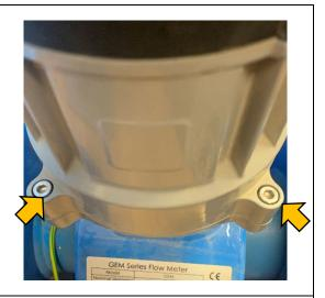
2. Remove the display cover by unlatching the three (3) clips that hold it to the battery cover. Two clips are shown, and the last clip is located on the opposite side.
