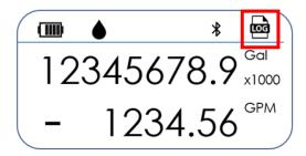
When the job totalizer is enabled, the totalizer will switch between displaying the totalizer 5 seconds and the job totalizer for 10 seconds.
